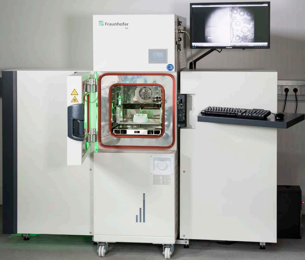
KLIMATOM performs measuring tasks in a non-contact, non-destructive manner
