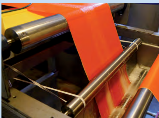
Equipment testing at German Project Partner TTR Ingenieurbüro für textile Verfahrenstechnik, featuring a vacuum extraction system from OptiVac AB, Sweden. (© STFI e.V.)
