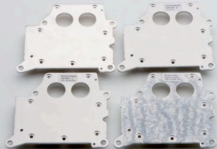
Different protection coatings after salt spray testing
