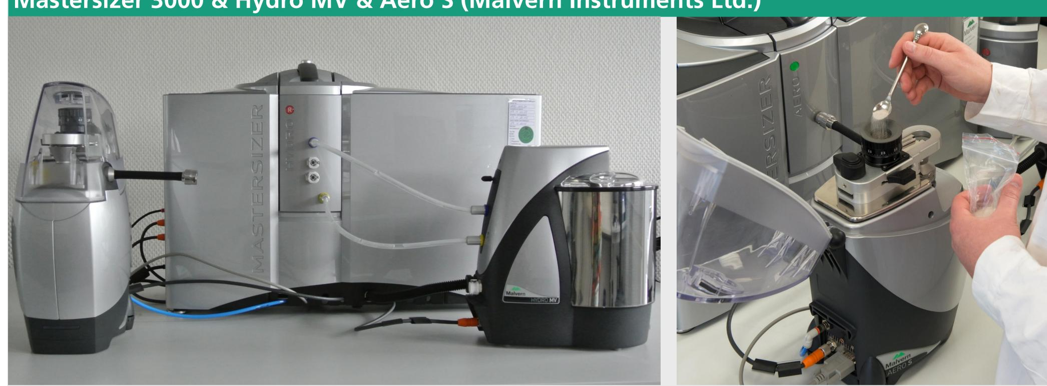
Laser diffraction  $\rightarrow$  particle size distribution The Mastersizer 3000 uses the technique of laser diffraction to measure the size of particles. It does this by measuring the intensity of light scattered as a laser beam passes through a dispersed particulate sample. This data is then analyzed via Mie or Fraunhofer scattering theory to calculate the size of the particles that created the scattering pattern.
