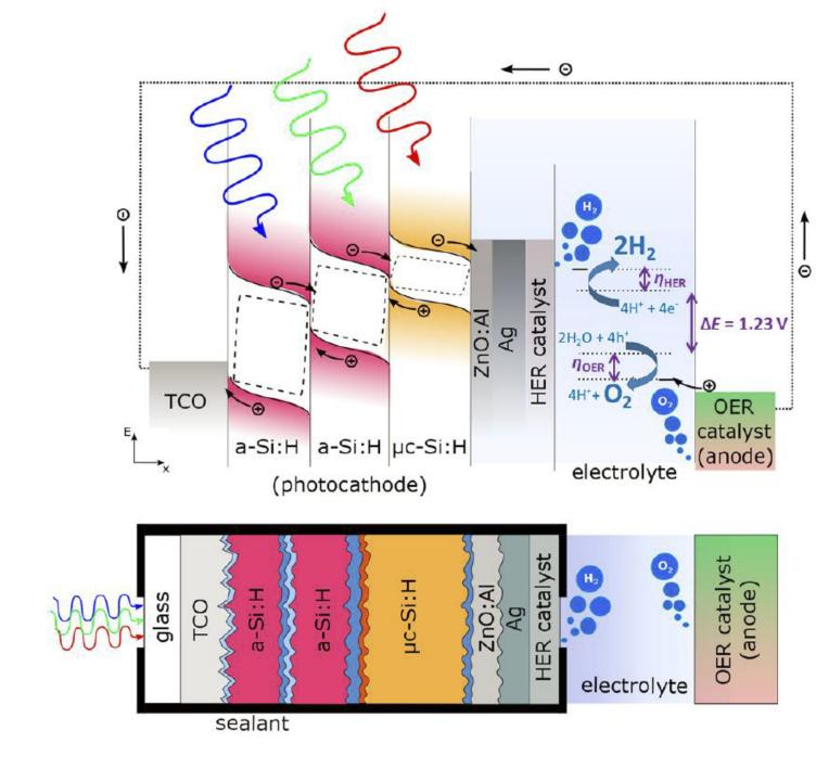
Solar cells:  $V_{OC} = 1.5 - 2.8 V$
