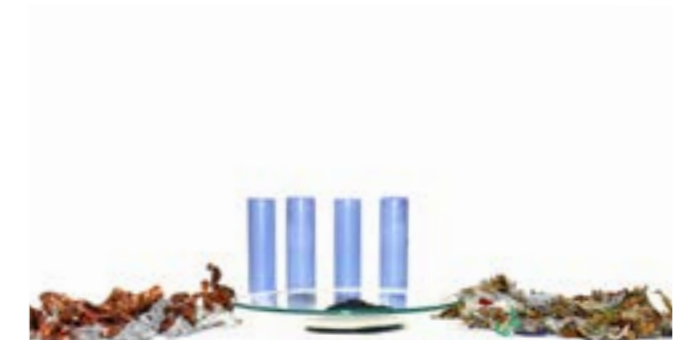
Picture: 18650 batteries as they are used in electric cars before and after the electro-hydraulic fragmentation
